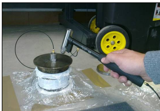
Figure 4. Detail of the experimental set-up for the mechanical test according to EN 29052-1.
