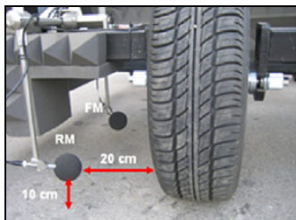
Figure 3. TiresonicMk4-LA 2 IC showing the semi-anechoic chamber for the close proximity measurements of the acoustic pavement behaviour, and a schematic drawing of the microphone positions.
