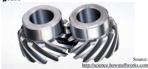
Figure A2: Example of helical gear
