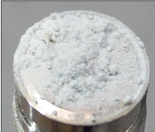
Fig. 11: heavy dust on the membrane
