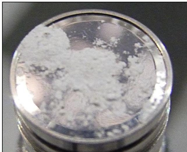
Fig. 9: light dust on the membrane
