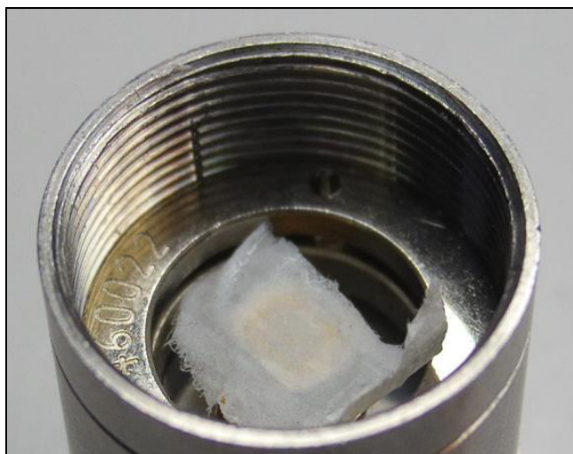
Fig. 19: humid paper on the inner pin of the microphone
