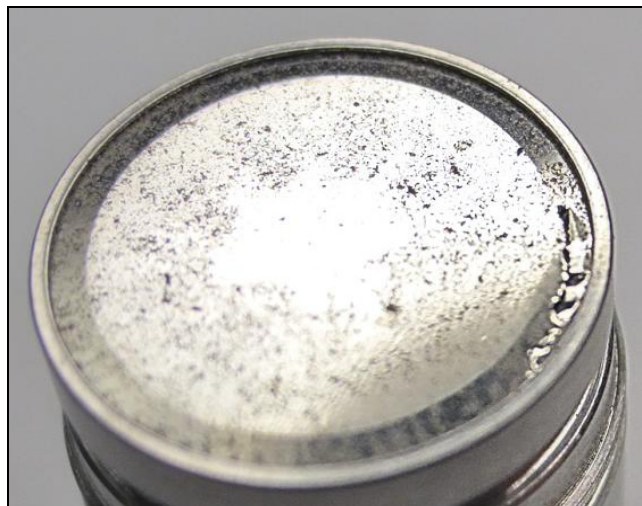
Fig. 17: large cut on the edge of the microphone
