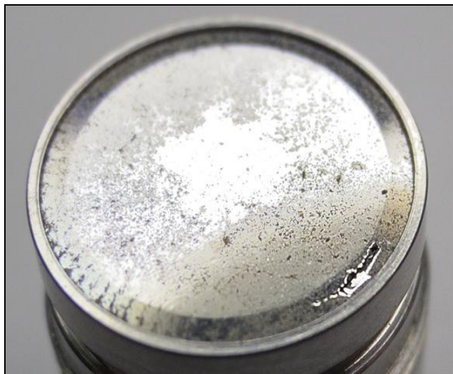
Fig. 15: small cut on the edge of the microphone
