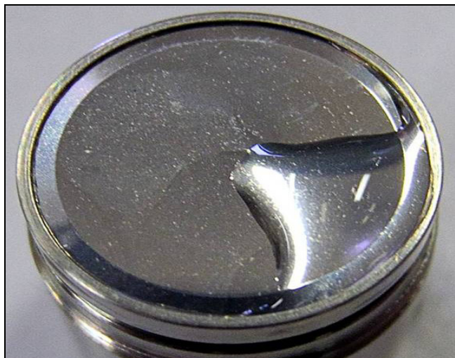
Fig. 7: water drop on the membrane
