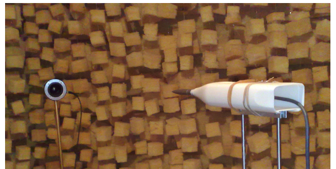
Fig. 6: Electro acoustic tests performed on 3D prints to validate the mechanical design of the body
