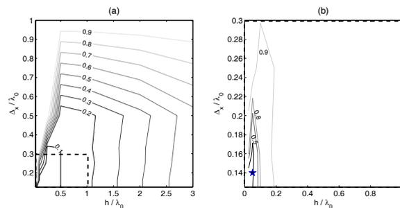
Figure 7: Reproduction error as a function of planes separation  $h$  and source separation  $\Delta_x$  – (a) Error  $\epsilon_{pp}^0$  calculated up to  $k_0$  and (b) Error  $\epsilon_{pp}^c$  calculated up to  $k_c$ .
