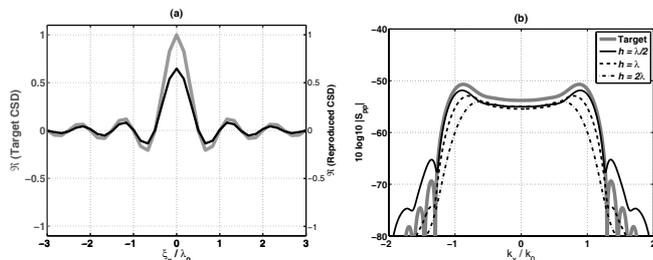
Figure 3: Reproduction of DAF – (a) Target CSD and reproduced CSD in the  $(\xi_x, 0)$  plane - (b) Target CSD wavenumber-spectrum and reproduced CSD wavenumber spectrum in the  $(k_x, 0)$  plane for various plane separations.
