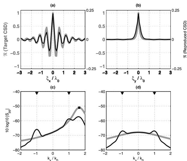
Figure 8: Subsonic TBL with  $\Delta_x = 0.14\lambda_0$  and  $h = \lambda_0/20$  – Target CSD and reproduced CSD in the  $(\xi_x, 0)$  plane (a) and  $(0, \xi_y)$  plane (b) – Target wavenumber-spectrum and reproduced wavenumber-frequency spectrum in the  $(k_x, 0)$  plane (c) and  $(0, k_y)$  plane (d).
