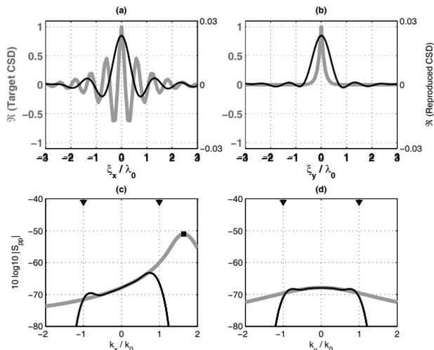
Figure 5: Subsonic TBL ( $U_\infty = 300$  m/s) – Target CSD (bold gray line) and reproduced CSD in the  $(\xi_x, 0)$  plane (a) and  $(0, \xi_y)$  plane (b) – Target CSD wavenumber spectrum and reproduced CSD wavenumber spectrum in the  $(k_x, 0)$  plane (c) and  $(0, k_y)$  plane (d).
