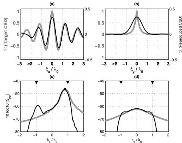
Figure 4: Supersonic TBL ( $U_\infty = 600$  m/s) – Target CSD (bold gray line) and reproduced CSD in the  $(\xi_x, 0)$  plane (a) and  $(0, \xi_y)$  plane (b) – Target CSD wavenumber spectrum and reproduced CSD wavenumber spectrum in the  $(k_x, 0)$  plane (c) and  $(0, k_y)$  plane (d).
