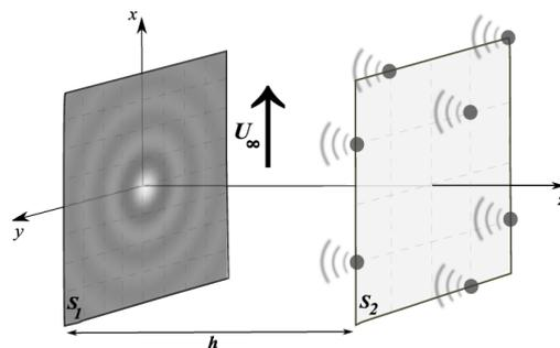
Figure 1: Problem geometry and coordinate system – The free-flow direction is indicated by the bold vertical arrow for the TBL case ( $U_\infty$  is the free-flow speed) –  $h$  is the distance separating the two planes – Illustrated CSD on plane  $S_1$  corresponds to a DAF.
