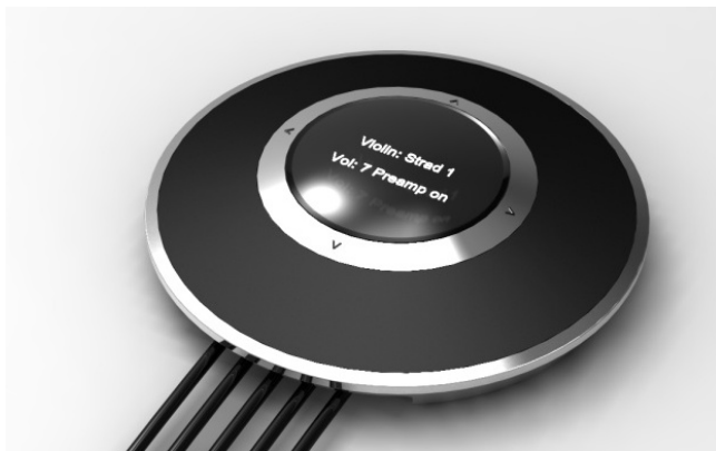
Figure 5. Violin body response emulator hardware.
