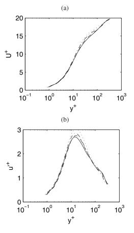
Figure 3: Grid convergence in the *x* direction: (a) mean, and (b) rms streamwise velocities. ..... Gdx1 ( $\Delta x^+ = 45$ ),  $- \cdot - \cdot Gdx2 (\Delta x^+ = 35), - - - Gdx3 (\Delta x^+ = 30),$ Gdx4 ( $\Delta x^+ = 15$ ).
