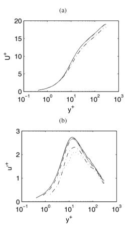
Figure 1: Grid convergence in the y direction: (a) mean, and (b) rms streamwise velocities. ..... Gdy1 ( $\Delta y_w^+ = 3.7$ ), ---- Gdy2 ( $\Delta y_w^+ = 1.9$ ), --- Gdy3 ( $\Delta y_w^+ = 0.95$ ), Gdy4 ( $\Delta y_w^+ = 0.47$ ), Gdy3 ( $\Delta y_w^+ = 0.95$ ) using the semi-implicit time integration scheme (SIRK)
