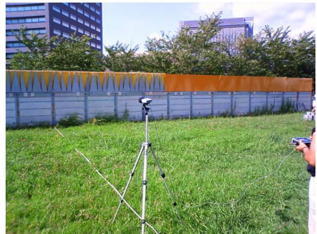
Fig. 6 Field measurement. Receiving positions are covered by flat grass. Left and right half of the barrier are consist of M-shaped and flat top edge, respectively.
