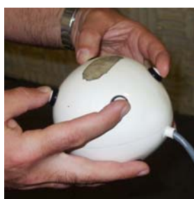
Figure 3: Pointing device used by the subject (sphere with eight buttons) for localization response
