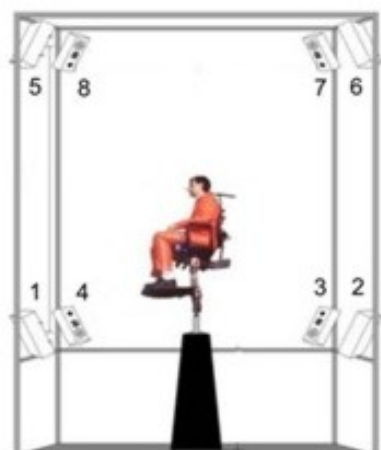
Figure 2: Representation of the arrangement of the semi-anechoic chamber for 3D localization of sound sources
