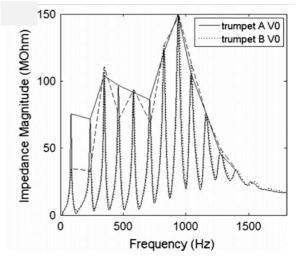
Figure 3: Input impedance of the two trumpets when no valve is pressed down
