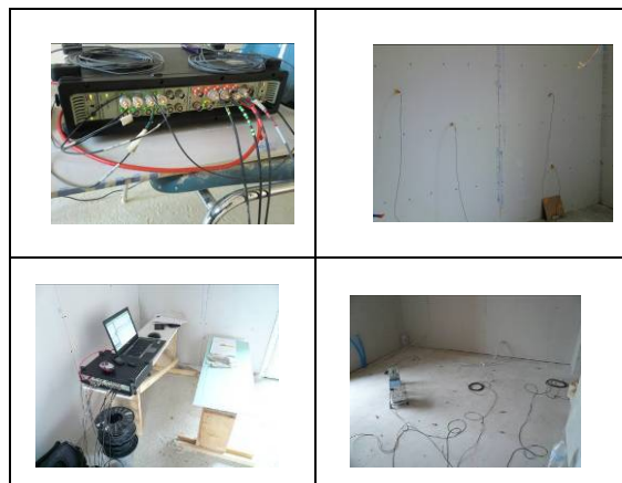
Figure 4: Vibration level difference in situ measurements
