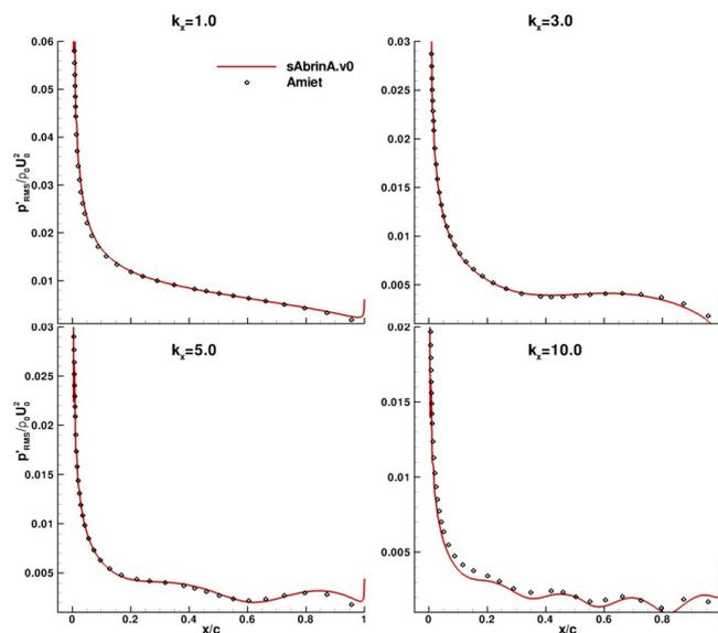
Figure 1: RMS wall pressure for  $k_x = 1, 2, 5$  and  $10$
