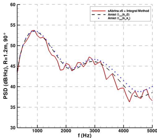
Figure 7: Predicted PSD at  $R_{obs} = 1.2$  m and 90°
