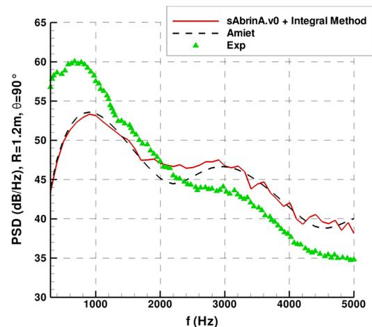
Figure 8: PSD at  $R_{obs} = 1.2$  m and 90° for the baseline case
