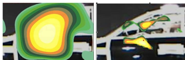
Fig. 5: Sound Intensity maps based on beamforming measurements in a wind tunnel. Left: delay and sum method. Right: Refined beamforming method.
