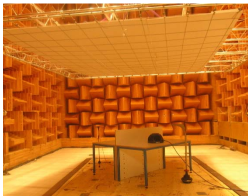
Figure 7: View of the measurement set-up with a reflective ceiling and a screen height of 1.10 m
