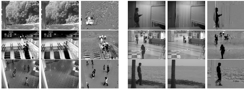
Fig. 4. I2R dataset. From left to right (split in two columns): The original image, the background model and their difference.
