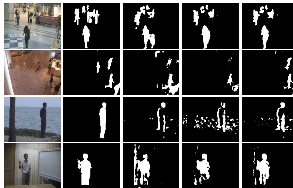
Fig. 3. Experimental results on the I2R dataset. From left to right: original image, ground truth, RSL, IALM, Fast-LSADM. From top to bottom: airport (2926), shopping mall (1980), water surface (1594), curtain (23257).
