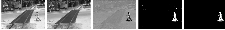
Fig. 1: Original image (309), low-rank matrix L (background), sparse matrix S (foreground), foreground mask, ground truth.
