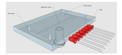
Figure 1. Schematic representation of a transparent (PDMS-on-glass) microfluidic device with LEDs for dark field illumination. The LED light is coupled into the PDMS which then acts as a light guide. Scattered light, as well as fluorescence are observed through the glass substrate using a microscope objective.
