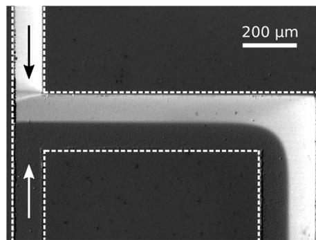
Figure 3. RLS image of a fluidic T-junction (green LED illumination), where flows of water (white arrow) and a suspension of AuBBI-50nm (black arrow) join. The exposure time was 10 seconds. A background image of a channel containing only water was subtracted. For clarity, the boundaries of the fluidic channels are indicated using dashed lines. Flow rate was  $1 \mu\text{min}^{-1}$  at each input. The LEDs for illumination are situated at the right from the image.
