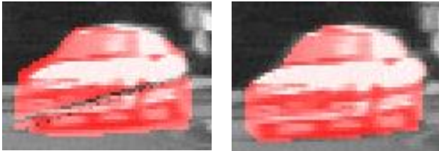
Fig 8: First image gives the result obtained using only motion model, second image give the result obtained after the refinement by graph cuts.
