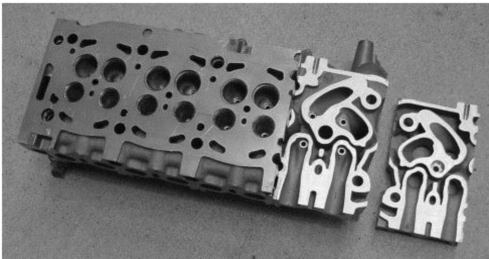
Fig. 1. The PSA diesel engine cylinder head. The upper surface is the engine block mating surface. The right end of the cylinder head has been sectioned via a horizontal cut.
