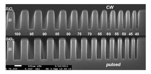
Fig. 28. Array of Si trenches with various widths etched in silicon with  $SiO_2$  hard-mask in HBr/O<sub>2</sub> plasma in CW and synchronous pulsing mode at 1 kHz 20% duty cycle.
