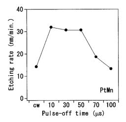
Fig. 18. Etch rate of PtMn in a Cl<sub>2</sub> (50 sccm, 2.025 mTorr, 1000 W) ECR plasma utilizing a 600 kHz RF bias power of 100 W as a function of afterglow time. The active-glow time of the plasma is fixed at  $30 \,\mu$ s. Reprinted with permission from S. Kumagai, T. Shiraiwa, and S. Samukawa, J. Vac. Sci. Technol. A **22**, 1093 (2004). Copyright 2004, American Vacuum Society.
