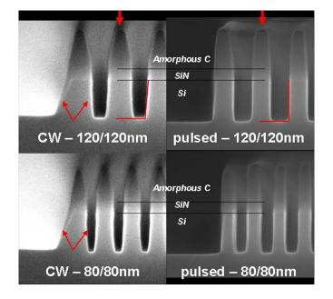
Fig. 26. (Color online) 120 nm-wide with space of 120 and 80 nm—wide with a space of 80 nm trenches etched in silicon in optimized HBr/O<sub>2</sub> plasma for both CW and synchronous pulsing modes.
