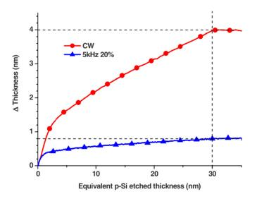
Fig. 24. (Color online) Damage penetration measured by kinetic *in situ* ellipsometry as a function of equivalent poly-Si etched thickness in CW and synchronous pulsing mode at 5 kHz and 20% duty cycle. Reprinted with permission from C. Petit-Etienne *et al.*, J. Vac. Sci. Technol. B **28**, 926 (2010). Copyright 2010, American Vacuum Society.
