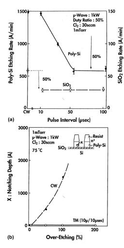
Fig. 14. (a) Etch rates of poly-Si and SiO<sub>2</sub> in Cl<sub>2</sub> (30 sccm, 1 mTorr, 1 kW) microwave plasma as a function of the pulse duration for a constant 50% duty cycle. (b) Notch depth at the foot of phosphorus-doped poly-Si as a function of over-etching time under CW and pulsed (50 kHz, 50% duty cycle) conditions in Cl<sub>2</sub> (30 sccm, 1 mTorr, 1 kW) microwave plasma. Reprinted with permission from S. Samukawa and T. Mieno, Plasma Sources Sci. Technol. **5**, 132 (1996).
