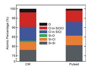
Fig. 22. (Color online) Surface composition of Si exposed to continuous wave and synchronous pulsed plasma at 1 kHz, 10% duty cycle. Si-Si contribution is not presented.
