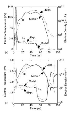
Fig. 8. Temporal dynamics of electron temperature and electron density in (a) absence of bias and (b) presence of bias in  $Cl_2$  ICP plasma with a peak power of 600 W pulsed at 10 kHz and a duty cycle of 50%. Sheath heating during the late after-glow leads to a capacitive discharge with higher electron temperature. Reprinted with permission from P. Subramonium and M. J. Kushner, Appl. Phys. Lett. **79**, 2145 (2001). Copyright 2001, American Institute of Physics.
