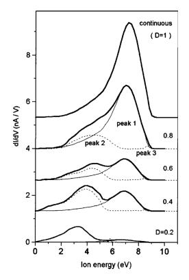
FIG. 7. Ion energy distribution functions in Ar microwave plasma with a peak power of 960 W pulsed at 1 kHz for varying duty cycles (*D*). Ion energies reflect the period of the pulse from which they originate depending on the duty cycle of the pulse. Reprinted with permission from O. Zabeida and L. Martinu, J. Appl. Phys. **85**, 6366 (1999). Copyright 1999, American Institute of Physics.
