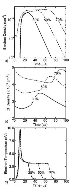
Fig. 6. Temporal dynamics of (a) electron density, (b)  $Cl^-$  density and (c) electron temperature in  $Cl_2$  plasma with a peak ICP power of 300 W pulsed at 10 kHz for duty cycles of 30%–70%. Reprinted with permission from P. Subramonium and M. J. Kushner, J. Appl. Phys. **96**, 82 (2004). Copyright 2004, American Institute of Physics.
