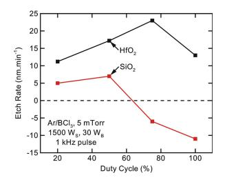
Fig. 25. (Color online) Time compensated etch rate of blanket  $SiO_2$  and  $HfO_2$  films as a function of the pulse duty cycle in etch-inhibitor regime (BCl<sub>3</sub>/Ar/5 mT/1500 Ws/30 Wb/1 kHz—synchronous pulsing).
