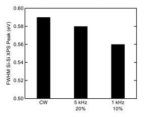
Fig. 23. FWHM of the Si-Si XPS peak measured by XPS at 45° photoelectron take-off angle for Si exposed to CW and synchronous pulsed  $\rm Cl_2$  plasma.
