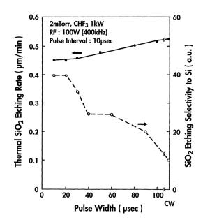
FIG. 19. SiO<sub>2</sub> etching rate and SiO<sub>2</sub>/Si selectivity as a function of activeglow duration for a fixed after-glow time of  $10 \,\mu s$  in a CHF<sub>3</sub> (20 sccm, 2 mTorr, 1000 W) ECR plasma utilizing a 400 kHz RF bias of 100 W on the wafer. Reprinted with permission from S. Samukawa, Jpn. J. Appl. Phys. **33**, 2133 (1994). Copyright 1994, The Japan Society of Applied Physics.
