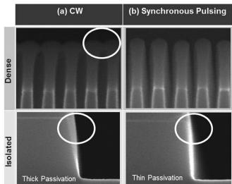
Fig. 27. Sub-20 nm trenches etched in  $HBr/O_2$  etch processes using (a) CW condition and (b) synchronous pulsed condition. Thin passivation layers are formed on the sidewalls of isolated lines under the pulsed mode while thicker passivation layers are formed in CW mode. Top clogging of trenches is observed in CW condition (from Ref. 114).
