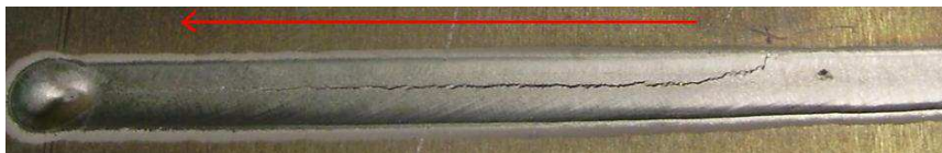
Fig. 1. Hot tearing in TIG welding.
