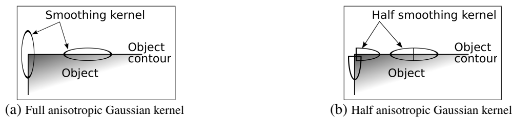
Figure 5: Anisotropic Gaussian kernels at linear portions of contours and at corners. Each ellipsoid represents a region where the major and minor axis are proportional to the standard deviation of the Gaussian kernel.
