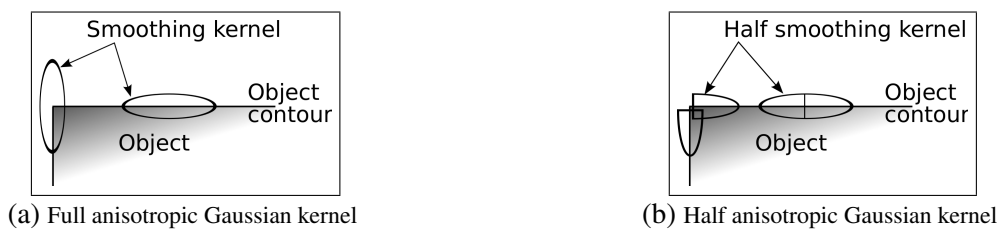
Figure 5: Anisotropic Gaussian kernels at linear portions of contours and at corners. Each ellipsoid represents a region where the major and minor axis are proportional to the standard deviation of the Gaussian kernel.
