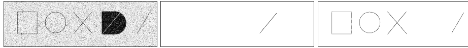
Fig. 9. Ridges and valleys detection on a noisy synthetic images ( 712 \times 220 ). Left to right: noisy image (uniform noise), ridges detection and valleys detection. \Delta\theta = 2 (degrees), \mu = 10 , \lambda_1 = 1 , \lambda_2 = 1.5 , \tau_L = 0.03 and \tau_H = 0.08 .
