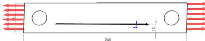
Figure 3: Specimen longitudinal tensile with fusion line TIG
