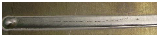
Figure 1: Hot tearing in TIG welding
