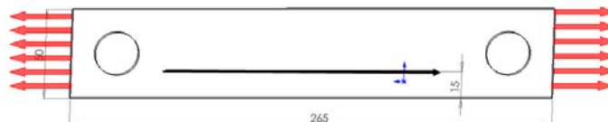
Figure 3: Specimen longitudinal tensile with fusion line TIG
