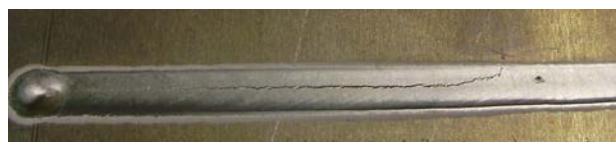
Figure 1: Hot tearing in TIG welding
