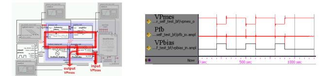
**Fig.7.** Self-test response in closed-loop. Pulses on the  $V_{Pbias}$  input generate Joule heating onto the resistance of the bolometer through the feedback shaping electronics so as to stimulate a response from the device. Presence or absence of pulses at the output, VPmes, indicates that the device is working
