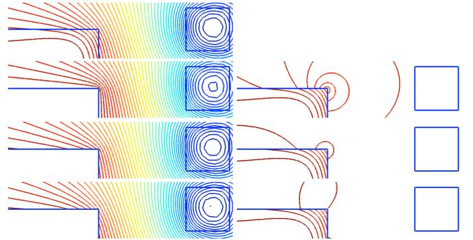
Fig. 1. Field lines near a conductor corner, from top to bottom: complete solution, left: PCBC, IBC, MIBC models, right: associated correction of each model; same scale for each figure pointing out the decrease of the required correction.
