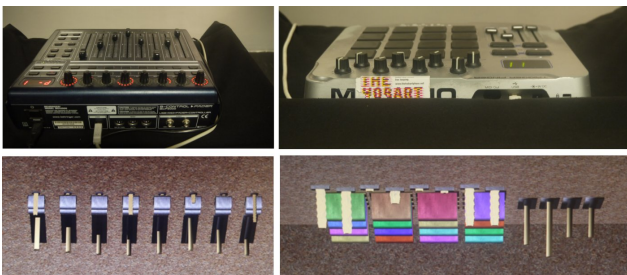
Figure 4: Two different controllers (seen from above) and the associated sets of virtual sensors extensions (seen from below)
