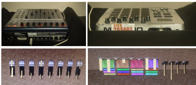
Figure 4: Two different controllers (seen from above) and the associated sets of virtual sensors extensions (seen from below)
