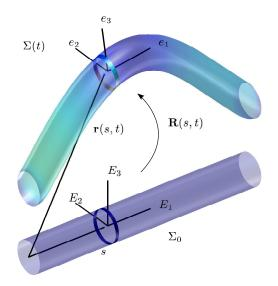
Fig. 1: Reference and current configuration of a beam. Each section, located at position *s* in the reference configuration  $\Sigma_0$ , is parametrized by a translation  $\mathbf{r}(s, t)$  and a rotation  $\mathbf{R}(s, t) \in SO_3$  in the current configuration  $\Sigma_t$ .
