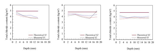
Figure 2: Differences between theoretical and measured chloride profiles for three specimens (with the values reported by [32]).
