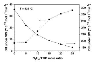
Fig. 6. Photocatalytic decomposition rate of Orange G solutions (10 ppm) using UV and VIS (>400 nm) light by N-doped TiO<sub>2</sub> ( $\sim$ 300 nm) layers grown on stainless steel at 425 °C, using various N<sub>2</sub>H<sub>4</sub>/TTIP mole ratios.
