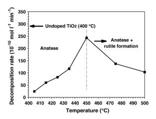
Fig. 3. Photocatalytic decomposition rate of Orange G solutions (10 ppm) under UV irradiation using N-doped TiO<sub>2</sub> layers ( $\sim$  300 nm thick) grown on stainless steel at various temperatures, using N<sub>2</sub>H<sub>4</sub>/TTIP mole ratio R=25. The TTIP mole fraction was 0.01%. The rate for undoped anatase (R=0) grown at 400 °C is given as reference.
