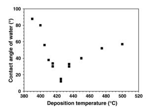
Fig. 5. Variation of the contact angle of water for various N-doped  $TiO_2$  films grown on stainless steel at various temperature using TTIP conc.=0.01% and  $N_2H_4/TTIP$ =25. The film thickness was approximately 275 nm. Measurements were made under the day light of the lab without additional UV or Vis irradiation.
