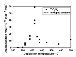
Fig. 4. Photocatalytic decomposition rate of Orange G solutions (10 ppm) under VIS irradiation (>400 nm) using N-doped  $TiO_2$  layers (~300 nm thick) grown on stainless steel at various temperatures using  $N_2H_4/TTIP$  mole ratio R=25. The rate for undoped anatase (R=0) grown at 400 °C is given as reference.
