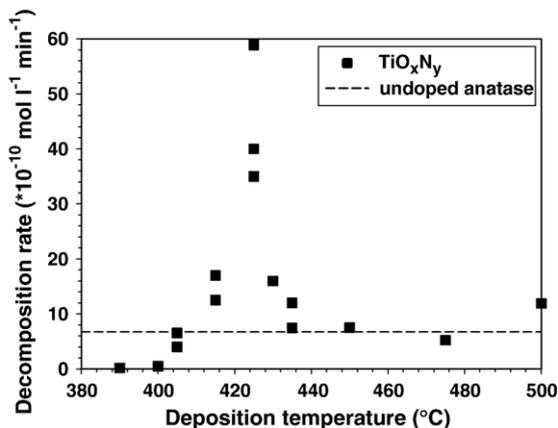
Fig. 4. Photocatalytic decomposition rate of Orange G solutions (10 ppm) under VIS irradiation (>400 nm) using N-doped TiO<sub>2</sub> layers (~300 nm thick) grown on stainless steel at various temperatures using N<sub>2</sub>H<sub>4</sub>/TTIP mole ratio  $R=25$ . The rate for undoped anatase ( $R=0$ ) grown at 400 °C is given as reference.
