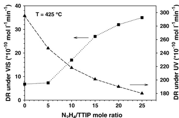
Fig. 6. Photocatalytic decomposition rate of Orange G solutions (10 ppm) using UV and VIS (>400 nm) light by N-doped TiO<sub>2</sub> (~300 nm) layers grown on stainless steel at 425 °C, using various N<sub>2</sub>H<sub>4</sub>/TTIP mole ratios.
