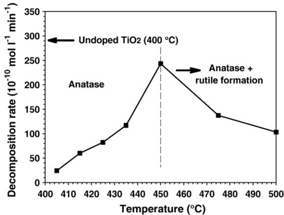
Fig. 3. Photocatalytic decomposition rate of Orange G solutions (10 ppm) under UV irradiation using N-doped TiO<sub>2</sub> layers (~300 nm thick) grown on stainless steel at various temperatures, using N<sub>2</sub>H<sub>4</sub>/TTIP mole ratio  $R=25$ . The TTIP mole fraction was 0.01%. The rate for undoped anatase ( $R=0$ ) grown at 400 °C is given as reference.
