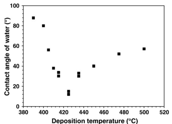
Fig. 5. Variation of the contact angle of water for various N-doped TiO<sub>2</sub> films grown on stainless steel at various temperature using TTIP conc.=0.01% and N<sub>2</sub>H<sub>4</sub>/TTIP=25. The film thickness was approximately 275 nm. Measurements were made under the day light of the lab without additional UV or Vis irradiation.
