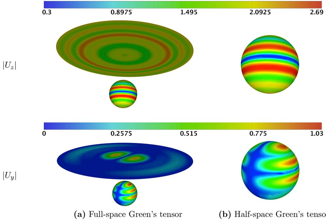
**Figure 5:** Comparison of the vertical and horizontal modulus of displacement obtained with (a) the full-space formulation (35) and (b) the half-space formulation (34).
