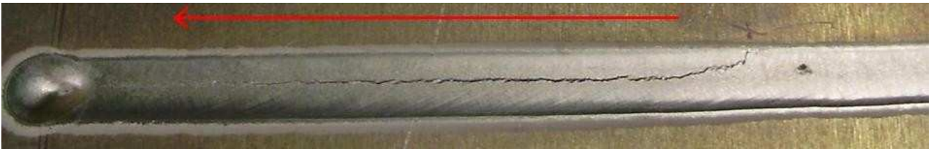
Figure 2: Autogeneous weld bead and crack location.
