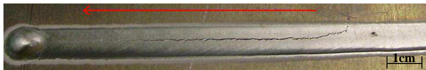
Fig. 1. Hot tearing in TIG welding.
