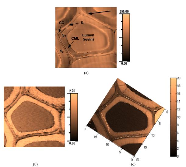
Figure 1: a) AFM topography (nm) of the sample surface in contact mode ( $20\times20~\mu m$ ): Embedding resin inside the lumen, CC-cell corner, CML-compound middle lamella,  $S_1$  and  $S_2$ -layers of the secondary wall. The arrow indicates the cutting direction. b) UFM amplitude (V) ( $T = 26.5^{\circ}C$ , RH = 45%,  $mc \approx 8.2\%$ ); c) Contact modulus (GPa) measured by RC-AFM ( $T = 21^{\circ}C$ , RH = 51%,  $mc \approx 9.2\%$ ).
