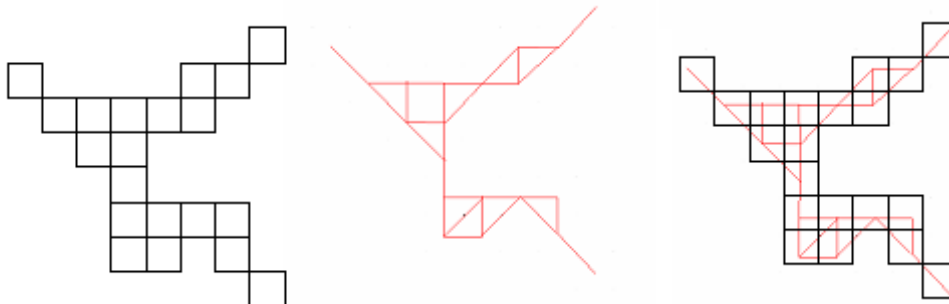
Figure 7: The initial volume (left), the corresponding Dijkstra tree (centre), and the two images superimposed (right). An example of a 2D case.
