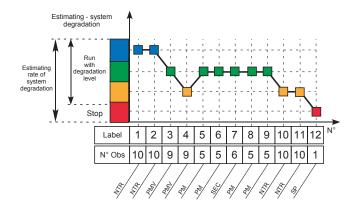
Fig. 2. Example of a degradation sequence of a process. The process starts at level 4. It becomes more and more degraded over time. After a Preventive Maintenance Visit (PMV), you can see that the degradation level increases on level 3. It decreases again until nothing is done (NTR: Nothing To Report) see label 10 and 11. Then, the process stops on label 12 (SP). PM is the symbol for Preventive Maintenance and SEC for a Security report.
