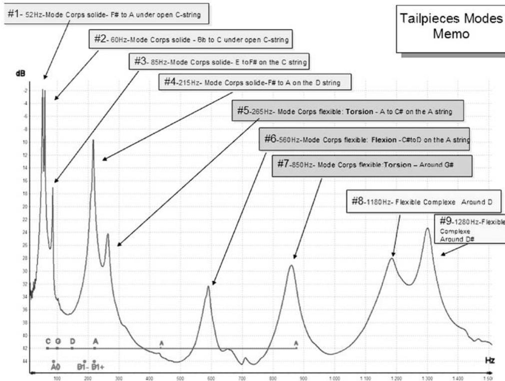
Fig. 6. Modes of cello tailpiece, strings, and range frequency of the body cello modes. Amplitude (dB)/Frequency (Hz).
