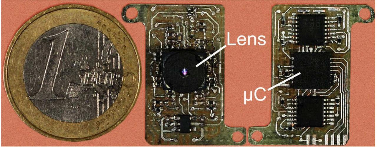
Fig. 1. Top view of the 1-gram microcontroller-based visual motion sensor (size:  $23.3 \times 12.3 \text{ mm}$ ) with its lens (focal length:  $2 \text{ mm}$ ) mounted on the one-dimensional 6-photosensor array, and bottom view of the PCB (thickness:  $0.4 \text{ mm}$ ) with its tiny low-power 16-bit  $\mu\text{C}$  (dsPIC from Microchip© Company).
