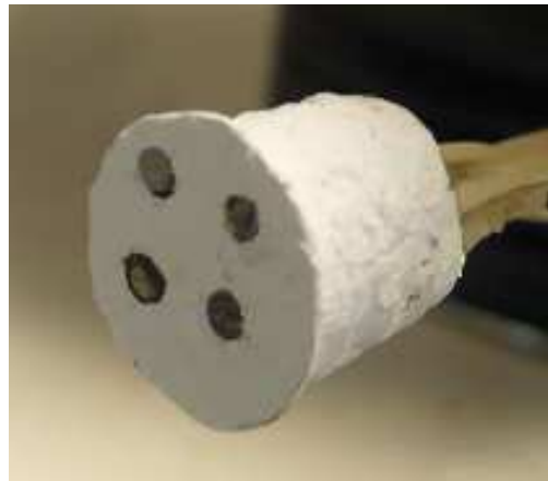
Figure 4. In house constructed resistivity probe
