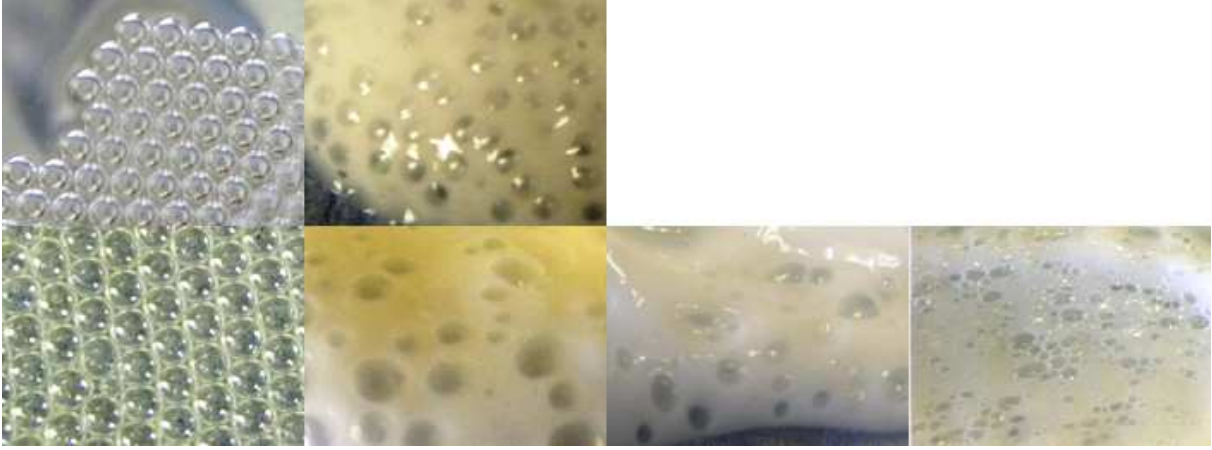
Fig. 10 Top: Pictures of an aqueous foam made of 1.6 mm diameter bubbles (left) and of a suspension of 1.6 mm bubbles made by mixing the foam with a 19 Pa yield stress emulsion (final interstitial emulsion yield stress: 9 Pa) [same scale for both images]. Bottom: Pictures of an aqueous foam made of 3 mm diameter bubbles (left) and of a suspension of 3 mm bubbles made by mixing the foam with (from left to right): a 19 Pa yield stress emulsion (final interstitial emulsion yield stress: 9 Pa), a 87 Pa yield stress emulsion (final interstitial emulsion yield stress: 19 Pa), and a 87 Pa yield stress emulsion (final interstitial emulsion yield stress: 72 Pa) [same scale for the 4 images].
