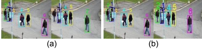
Fig. 3: Tracking results of SRC only with color feature (a) and SRC with feature integrating color and 2-dimensional coordinates (b). In (a), object 6 switches into object 2 after 13 frames due to similar appearance.
