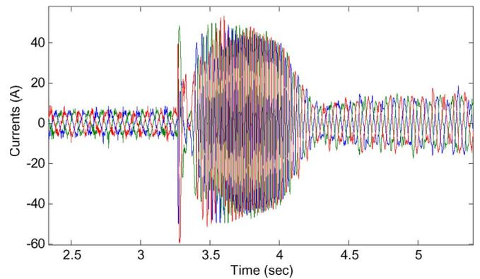
Fig. 13. Induction motor stator currents with load torque of 5.4 N · m.
