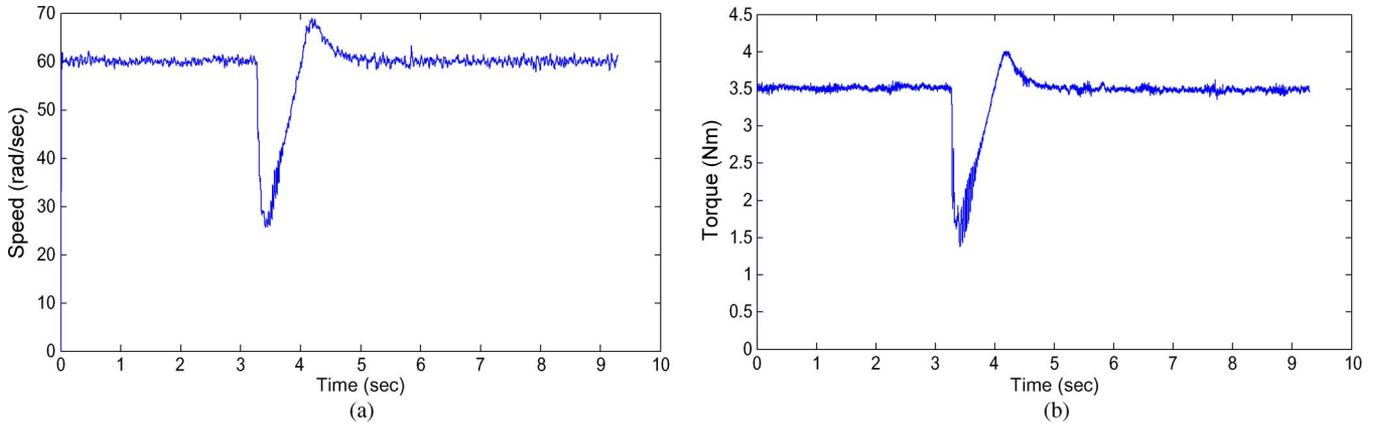
Fig. 14. Dynamics performances using the proposed reconfiguration mechanism with load torque of  $5.4 \text{ N} \cdot \text{m}$  load torque. (a) Induction motor speed. (b) Induction motor torque.
