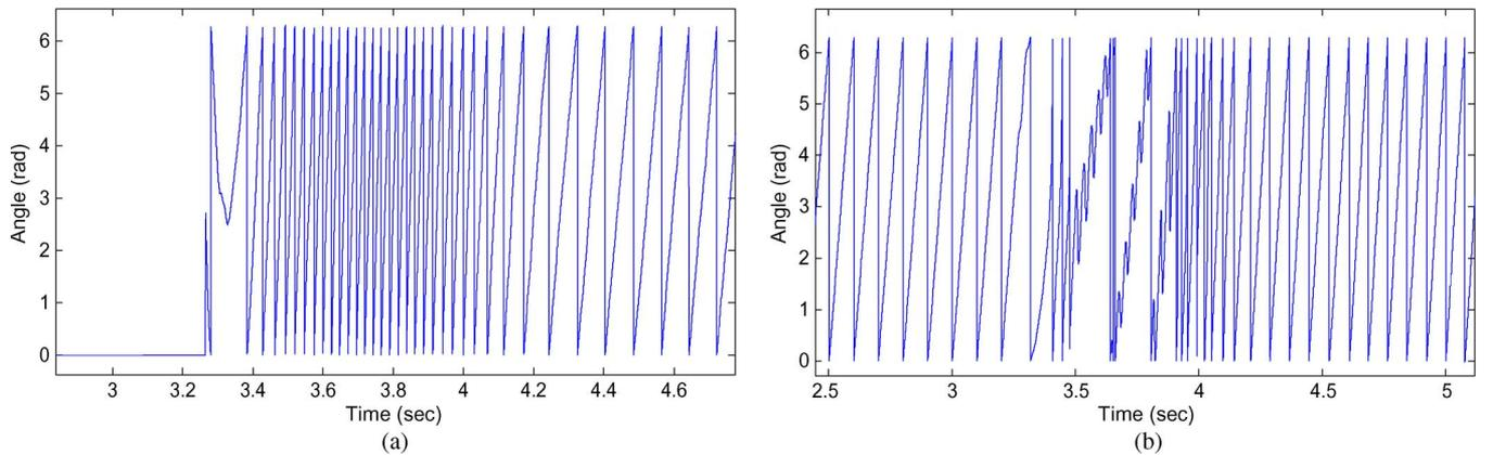
Fig. 12. Generated control angles with load torque of 5.4 N · m. (a) SCSR-generated control angle. (b) FTC control angle (with contribution from the two controllers).
