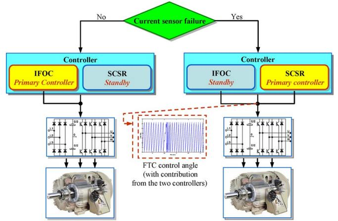
Fig. 7. Controller transition principle.
