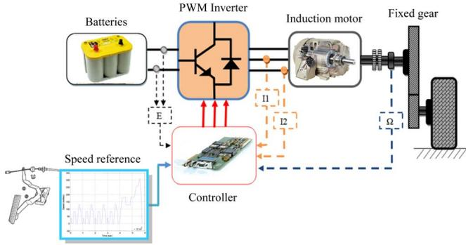
Fig. 1. Main components of an EV traction drive.
