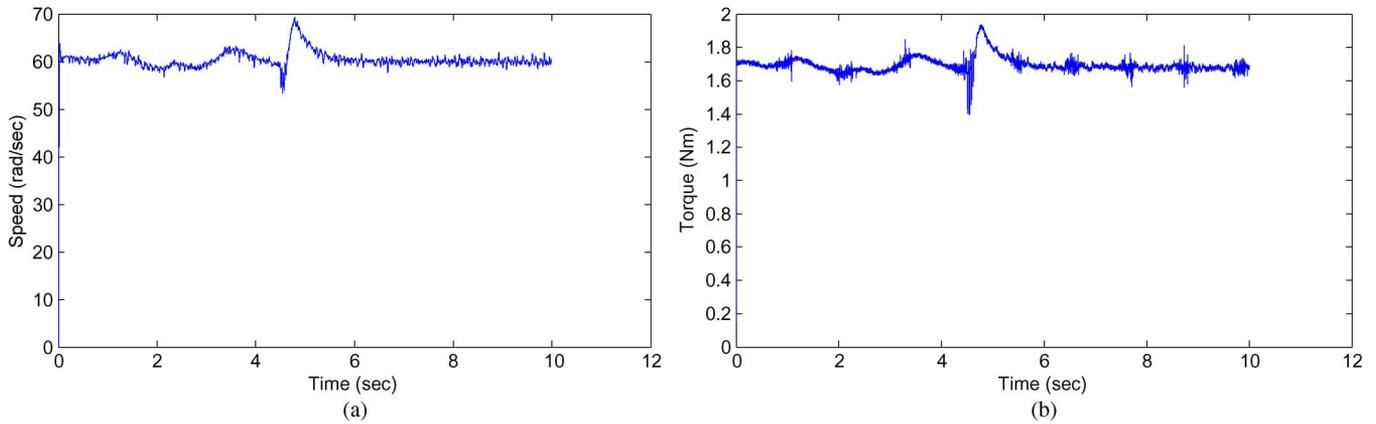
Fig. 11. Dynamics performances using the proposed reconfiguration mechanism with load torque of 2.6 N · m. (a) Induction motor speed. (b) Induction motor torque.
