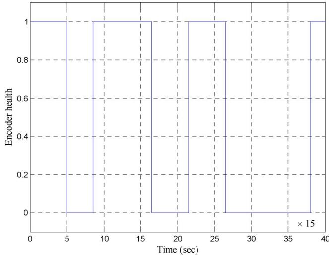
Fig. 7. Speed sensor simulated failures and recovery.
