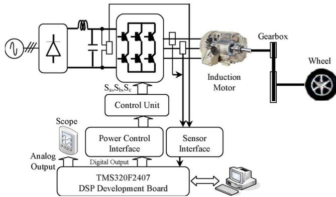
Fig. 12. View and schematic description of the experimental setup.
