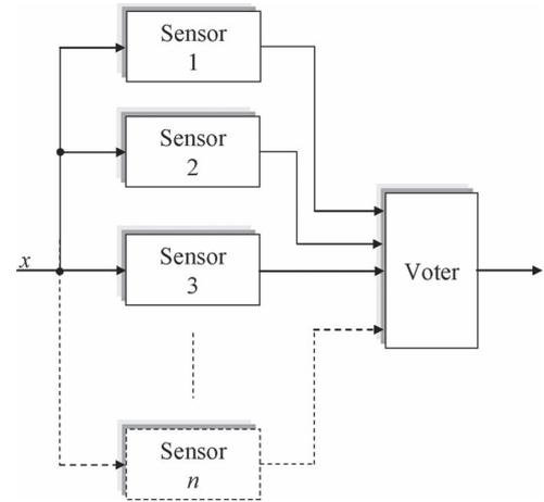
Fig. 5. Static redundancy.
