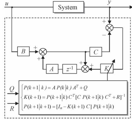
Fig. 3. Kalman filter recursive algorithm.
