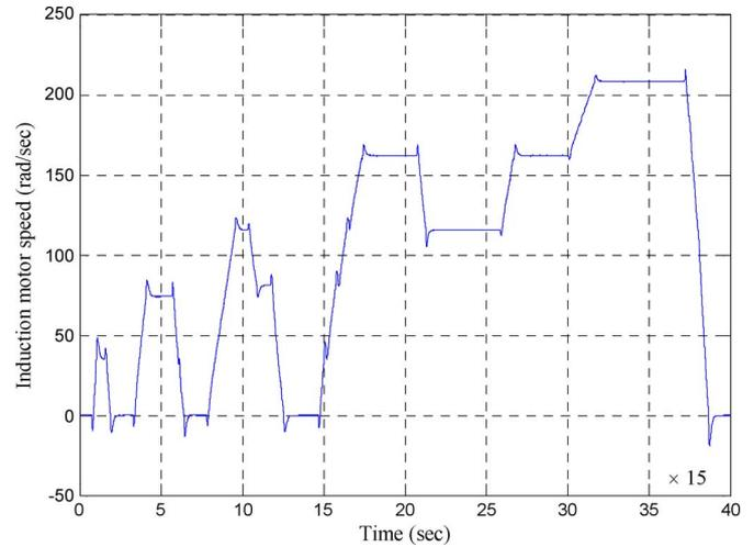
Fig. 9. EV induction-motor speed (ECE + URL).
